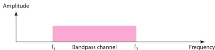
Figure 1.43 Bandwidth of a band pass channel
